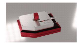
The ESPY31 enables quick and precise measurement of the piezoelectric  $d_{31}$  and  $d_{32}$  coefficients of piezoelectric polymer films or other soft piezoelectric materials such as fibres or membranes. It contains an integrated force measurement cell. It is a highly sensitive measuring device that can also be used to measure other electric properties, like P-E hysteresis or capacitance.
